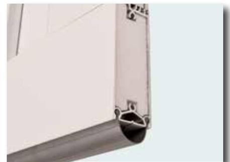
The bottom weather seal keeps out wind, rain, debris and other elements. Optional 3-layer sandwich construction with insulating polystyrene core increases energy savings (R-value 5.6)
