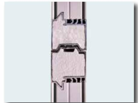
The Hörmann Infinity Classic 7800 is constructed with precisely engineered Tongue and Groove section joints that utilize an enclosed box type construction with a flexible gasket that reduces air infiltration creating a weather-tight seal.
